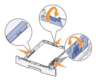
If you are loading legal or folio size paper, press down on the latch at the back of the tray and expand the tray until the extender locks into place.
